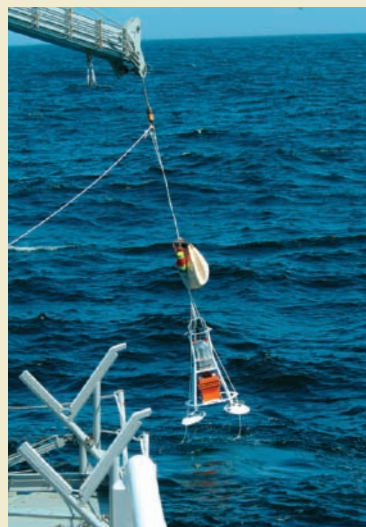
PAMS on Hoist
