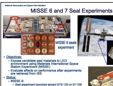
Mounted on ISS Columbus module for 9-12 mos.
