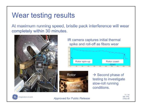
Wear testing setup at GE GR in Niskayuna, NY.
