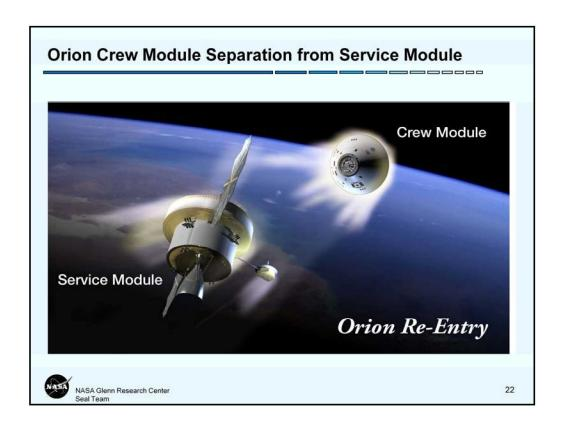
The Orion spacecraft is being designed to ferry astronauts either to the International Space Station or to the Moon. Upon return and during final stages of the mission, the Crew Module separates from the Service module and prepares to re-enter the Earth's atmosphere during which time extensive aeroheating occurs requiring a robust thermal protection system (TPS) and corresponding seals.
