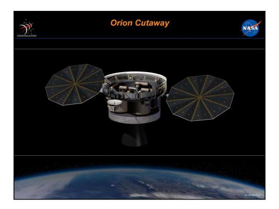
Orion will use 5.5m (18ft) in diameter radial UltraFlex solar arrays. Recent tests validated the UltraFlex array's acceleration capability, up to 2.7g, required for Orion's lunar missions. Smaller-scale arrays are powering NASA's Phoenix Lander that is on Mars.
