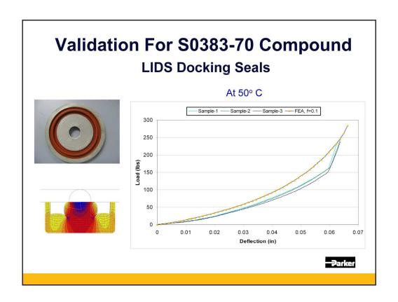
Axisymmetric analysis with thermal expansion. In FEA, the beat height at 50° C is about .066". However, the height of tested samples is about .060", possibly due to permanent set after previous loading.
