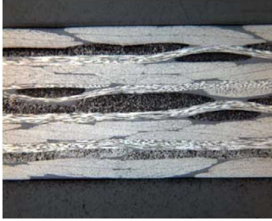
Figure 5 Photomicrographs of a-ODPA/3,4' -ODA/PEPA composites after post cured at 343 °C for 8 hrs
