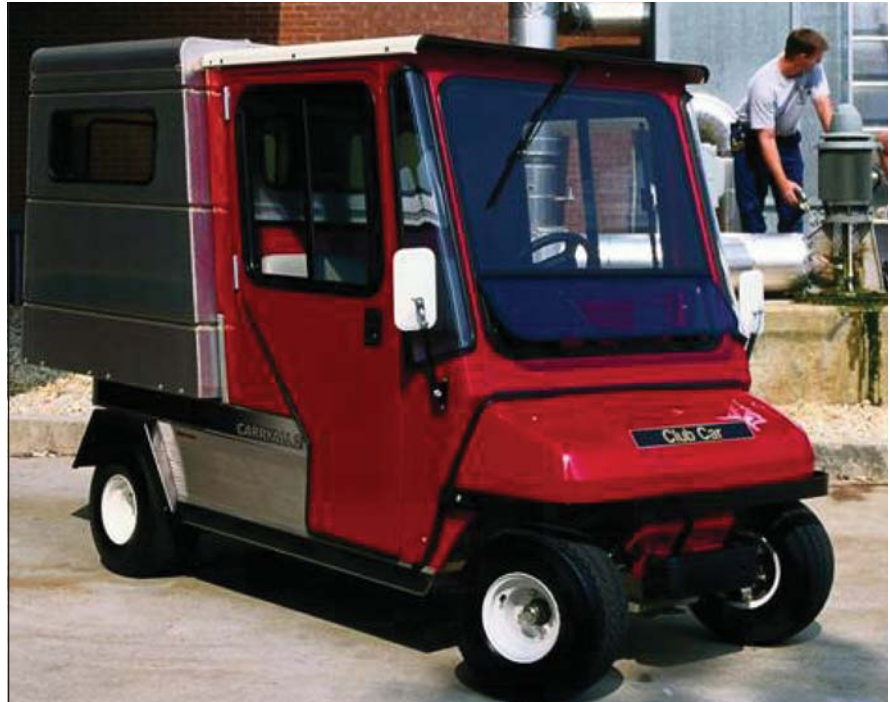
Figure 1. This Fuel-Cell-Powered Utility Vehicle has been used to demonstrate the practicability of hybrid power management.
