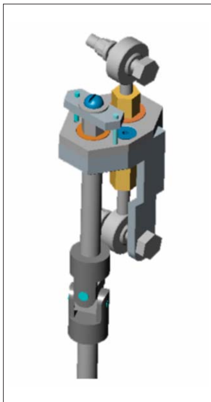
The Tool Assembly adjusts the length of the turnbuckle while it is still attached to the engine, eliminating the problem of removing and installing the actuator system back onto the engine.
