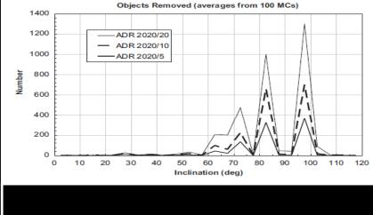
Positive results of Active Debris Removal by the removal of 5, 10, or 20 objects removed per year.
