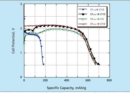
These **Discharge Curves** are typical of results of tests, at a temperature of -40 °C, of cells containing fully fluorinated ( $CF_{1.08}$ ) and sub-fluorinated ( $CF_{0.65}$ ) cathode materials. These tests were performed at a discharge rate of C/10 and C/5, as labeled. At a potential of 2 V, the  $CF_{0.65}$  cathodes exhibited over 3 times the specific capacity of the  $CF_{1.08}$  cathode.
