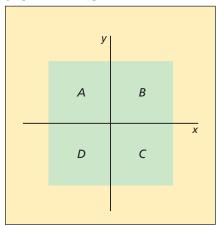
A **Square or Rectangular Array** of four photodetectors would provide indications of the x and ydisplacements of a star image from the origin, which would lie at the center of a coronagraph mask.
