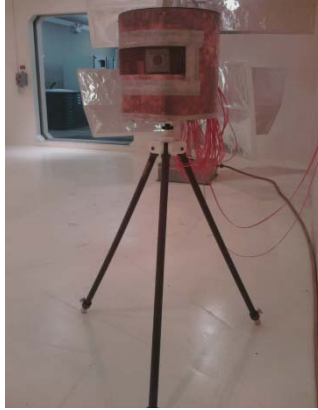
Figure 5-1: HIRF Laboratory portable camera in shielded enclosure.
