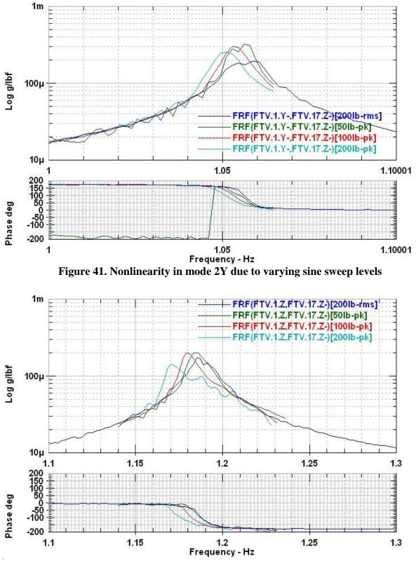
Figure 42. Nonlinearity in mode 2Z due to varying sine sweep levels
