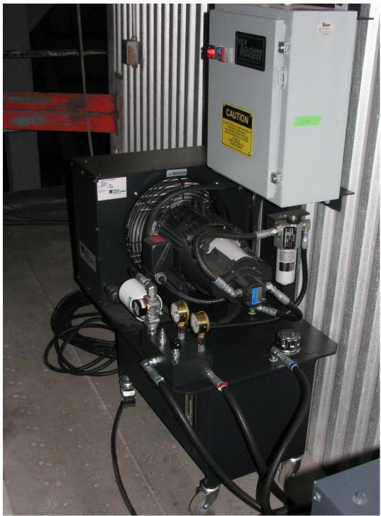
Figure 14. Hydraulic Power Supply.
