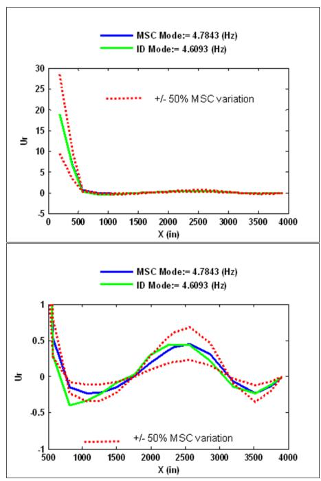
Figure 61. Comparison of mode shape deformation and nodal lines along sensor line for 4<sup>th</sup> Bending mode. Full vehicle (Top) and with LAS measurement points removed (Bottom).
