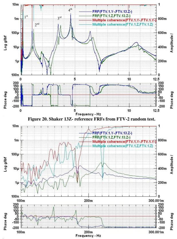
Figure 21. Shaker 13Z- low frequency for reference FRFs from FTV-2 random test.
