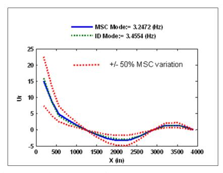
Figure 60. Comparison of mode shape deformation and nodal lines along sensor line for 3<sup>rd</sup> Bending mode.
