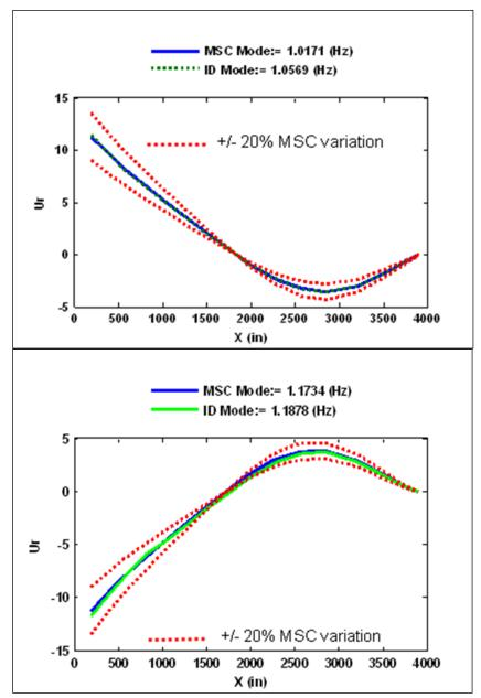
Figure 59. Comparison of mode shape deformation and nodal lines along sensor line for 2<sup>nd</sup> Bending Mode Y-Axis (Top) and Z-Axis (Bottom).
