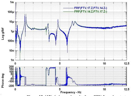
Figure 25. 135° shaker reciprocity from FTV-2 random test
