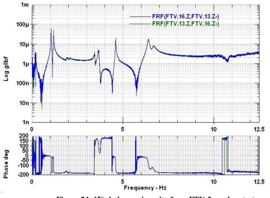
Figure 24. 45° shaker reciprocity from FTV-2 random test.
