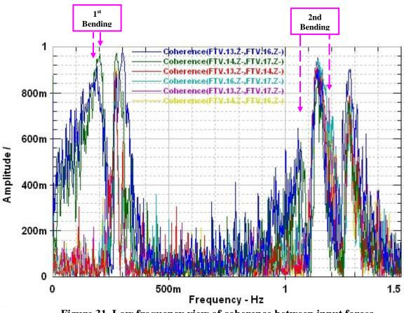
Figure 31. Low frequency view of coherence between input forces
