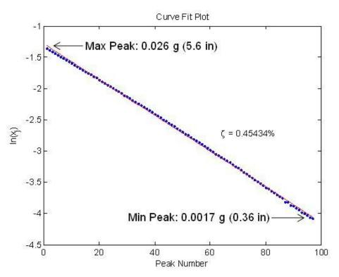
Figure 38. Fit of damping from first Z-direction free decay test (location 1Z)
