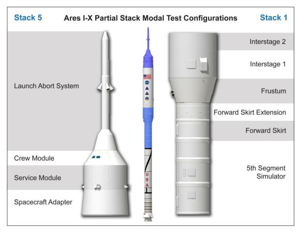
Figure 3. Ares I-X Subassembly Modal Test Configurations
