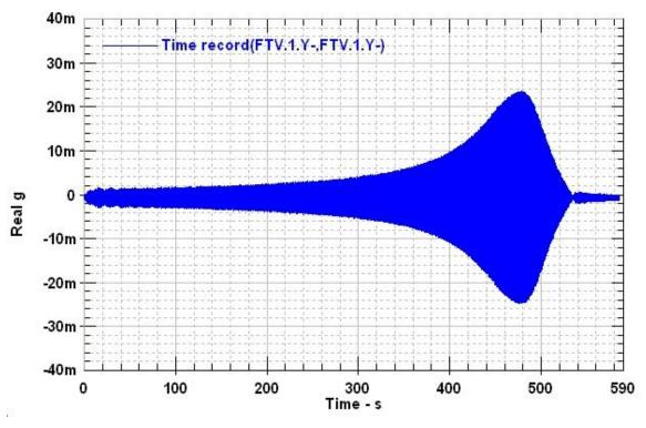
Figure 40. LAS Tip Acceleration for 100 lb-pk sine sweep of mode 2Y
