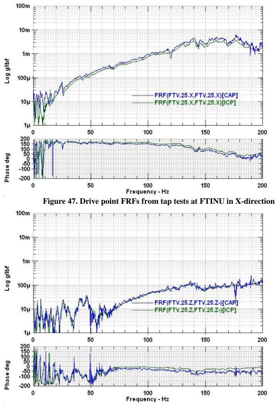
Figure 48. Drive point FRFs from tap tests at FTINU in radial direction
