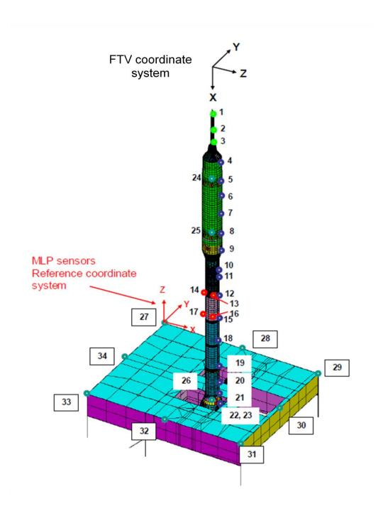
Figure 6. FTV on MLP sensor/shaker locations.
