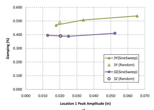
Figure 53. Amplitude dependence of 3<sup>rd</sup> bending mode damping estimates
