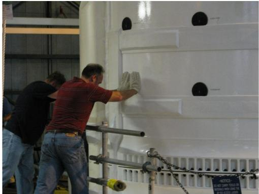
Figure 34. Manual excitation for 1<sup>st</sup> bending mode in Y-direction.
