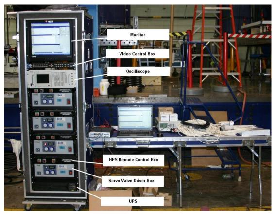
Figure 15. Hydraulic shaker equipment rack.
