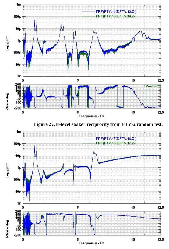
Figure 23. B-level shaker reciprocity from FTV-2 random test.
