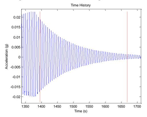
Figure 35. Third Y-direction free decay test time history (location 1Y)
