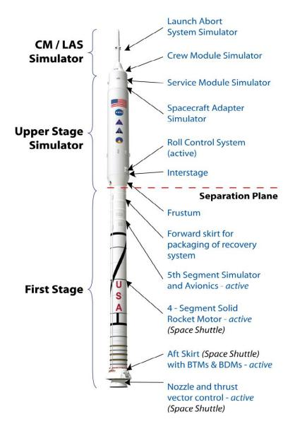
Figure 1. Ares I-X Flight Test Vehicle [1].
