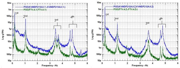
Figure 55. Comparison of pre-modal test (green) and on-pad (blue) ambient response for crew module accelerometers. Y-axis response (Left) and Z-axis response (Right).
