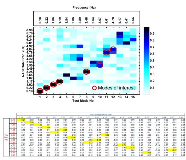
Figure 57. Cross-orthogonality matrix in graphical and table format.
