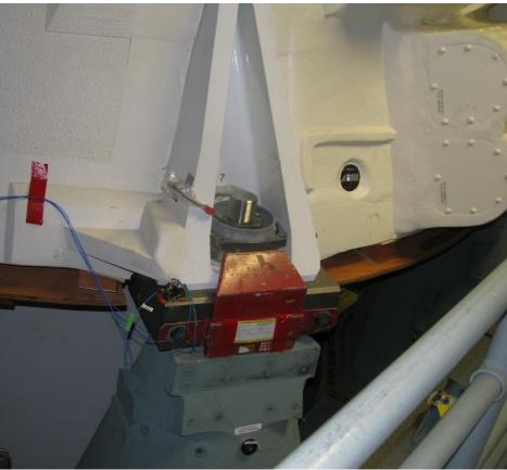
Figure 9. FTV to MLP attachment at Hold-down Post #7.
