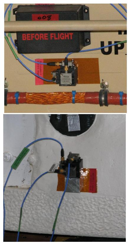
Figure 12. Typical accelerometer installations; (top) service module-location 4 interior and (bottom) aft skirt-location 23 exterior.
