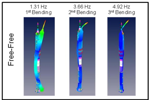
Figure 2. Free-free bending target modes.
