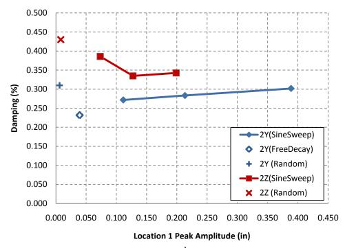
Figure 52. Amplitude dependence of 2<sup>nd</sup> bending mode damping estimates
