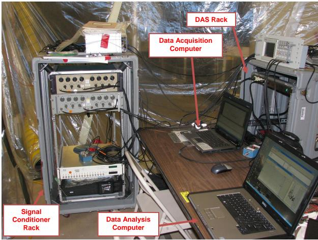
Figure 17. Signal conditioner and filter rack.
