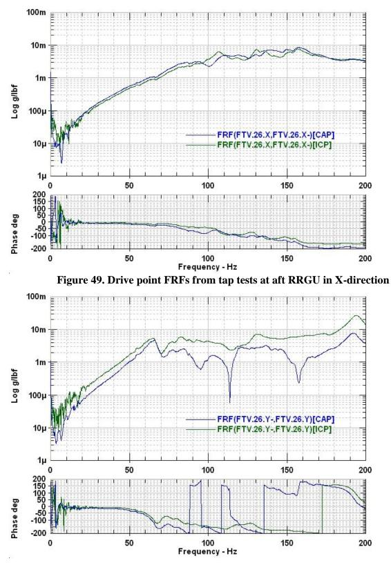
Figure 50. Drive point FRFs from tap tests at aft RRGU in radial direction
