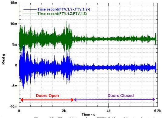
Figure 18. Time history from FTV-P10 ambient noise test.
