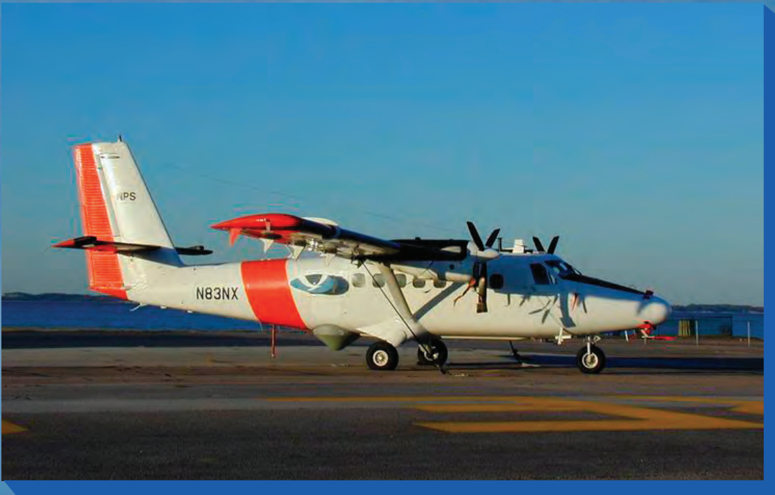
CIRPAS Twin Otter is non-pressurized turbo-prop, twin-engine aircraft.
