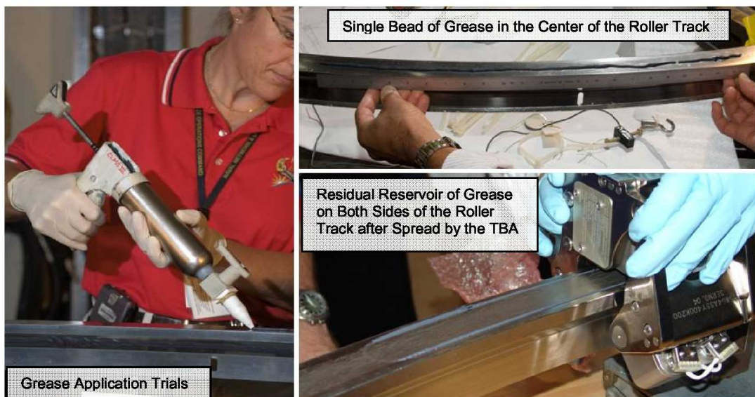
Figure 17. Final Grease Application Methods
