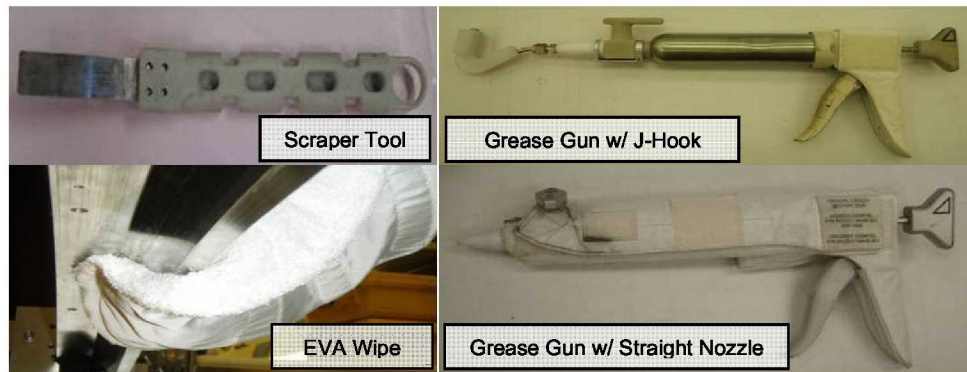
Figure 16. Tools used in SARJ Clean and Lube Operations
