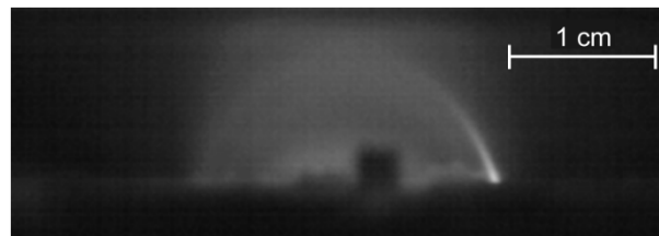
Figure 5.—Image of a cathode spot plume emanating from the electrode surface captured with a fast frame rate camera. The cathode spot is located on the electrode surface, and the plume is vaporized steel.
