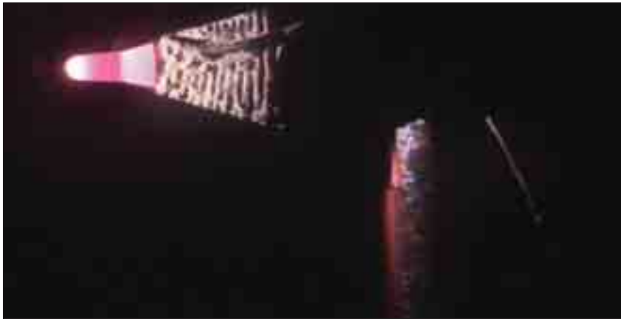
Figure 2. A UHTC Cone is shown during testing in the NASA Ames Arc Jet facility. Surface temperatures on the tip of the cone model exceeded 2,000°C during this test.
