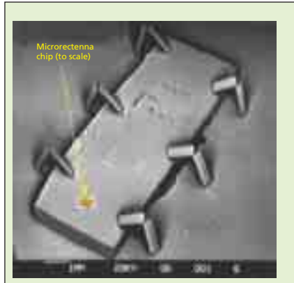
Figure 1. A Synthetic Image of the Microrectenna described in the text is here superimposed, to scale, on a real scanning electron micrograph of an insectlike microrobot. The underlying idea is to use the microrectenna to convert power from an incident 2.5-GHz radio beam to drive the robot and/or to charge its microbattery.
