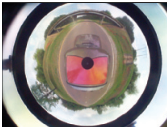
Figure 1. A Prototype PDS Mounted on Top of a Car acquired a panoramic image of the surroundings.
