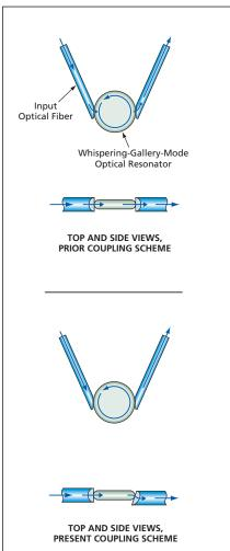
These Two Input/Output Coupling Schemes differ in the position and orientation of the output optical fiber. In the present scheme, the output fiber is tilted to reduce coupling to the fundamental modes of the resonator.
