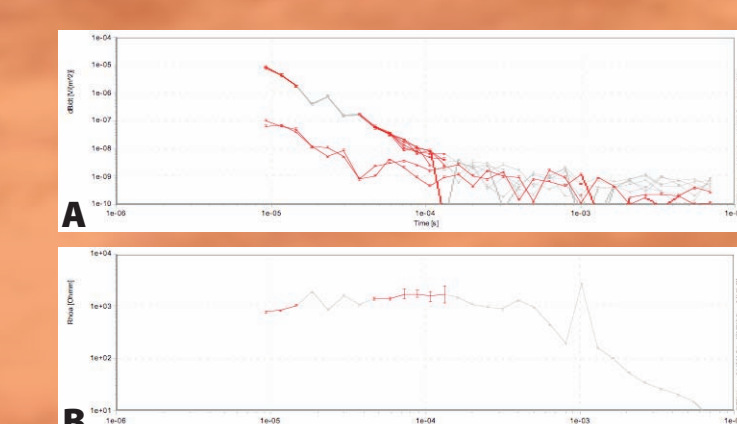
A) Un-normalized dB/dt data from station A5 (center of loop A). Lower two curves are noise sweeps. B) Average apparent resistivity at station A5.
