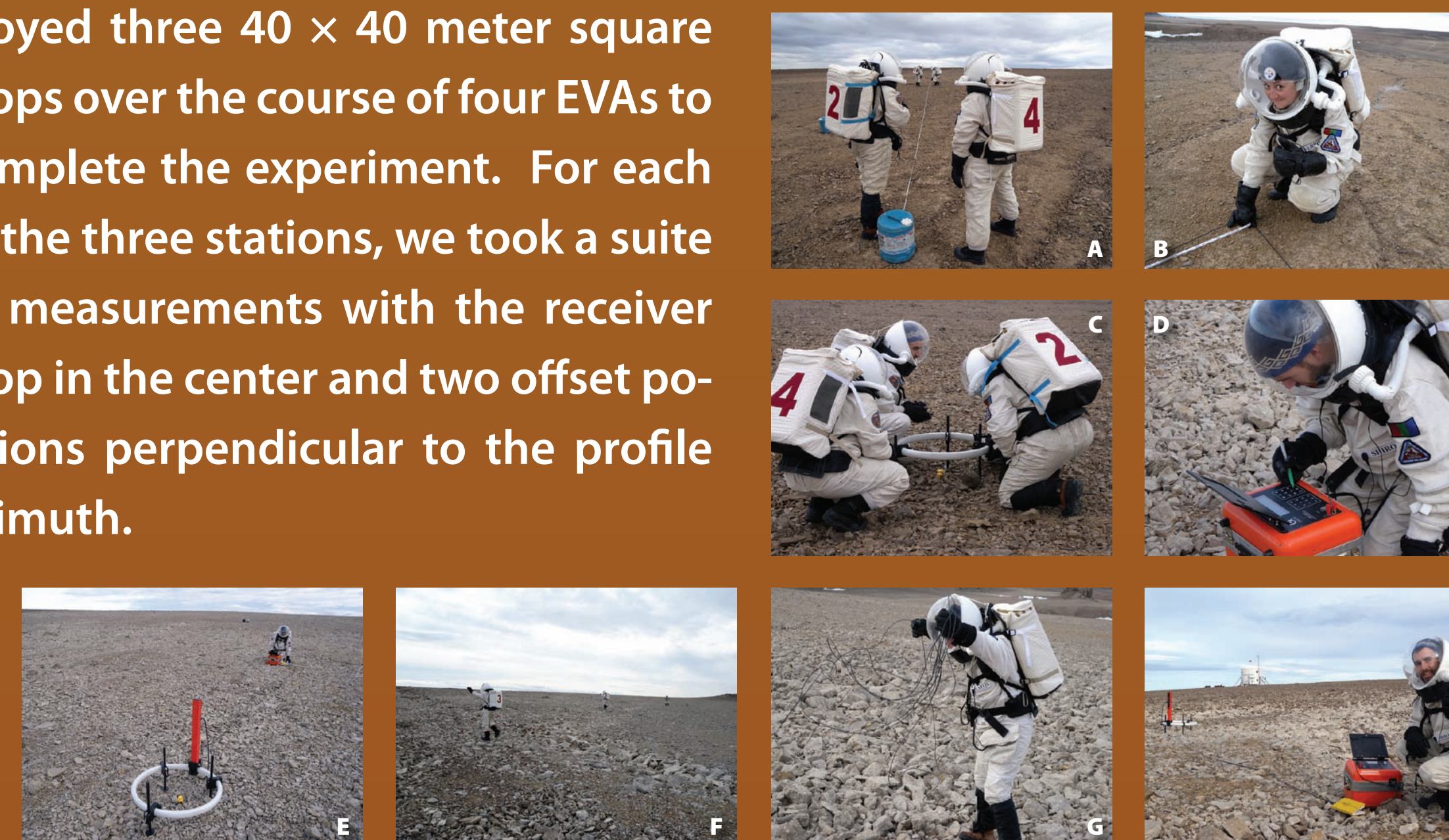
A) Survey the profile. B) Lay out the square transmitter loop. C) Set up the receiver coil. D) Configure the receiver. E) Take sounding measurements. F) Move the loop. G) Untangle the wires. H) Repeat at each station.
