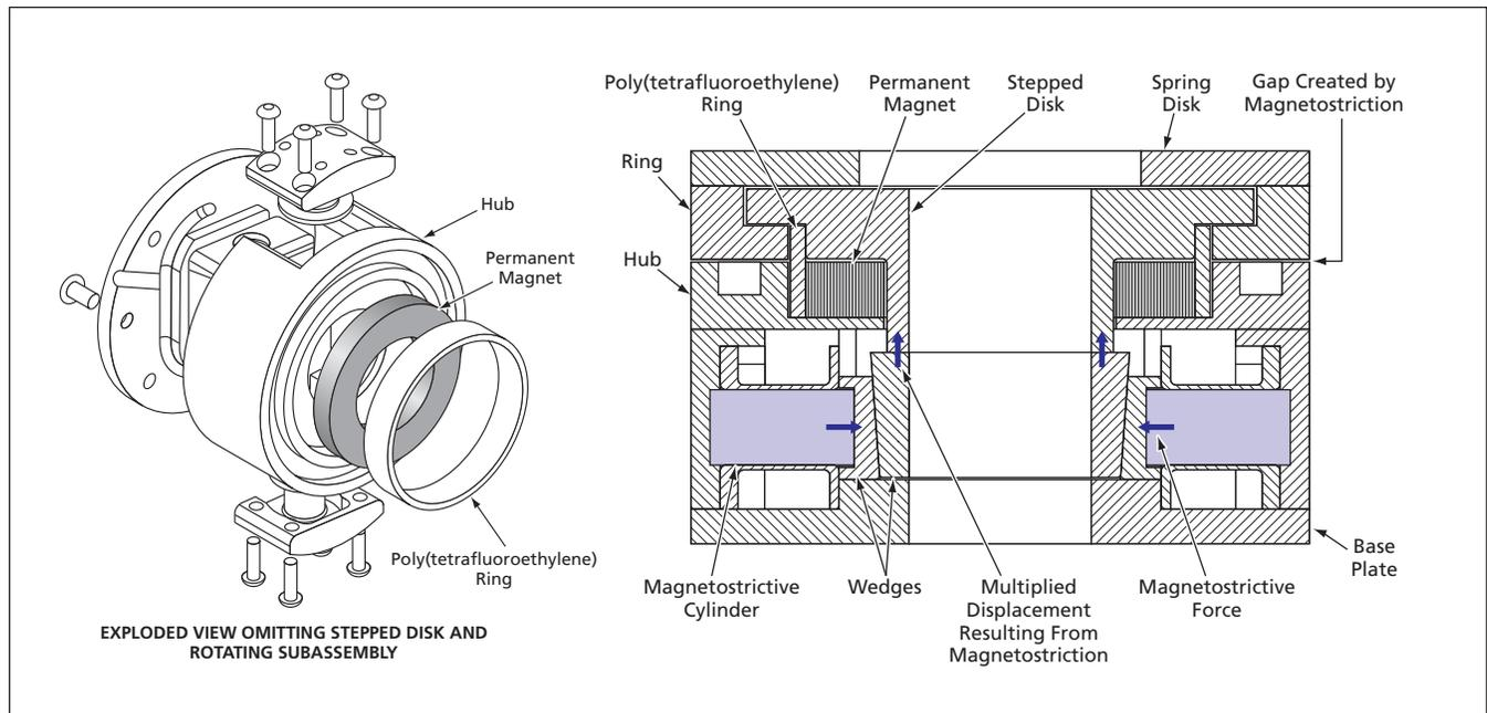
In the **Magnetostrictive Brake**, a large braking force would be generated by the permanent magnet. When power was supplied to electromagnet coils (not shown) surrounding the magnetostrictive cylinders in the solenoid assemblies, the resulting magnetostrictive strain would be converted to a force and displacement that would oppose the braking force.
