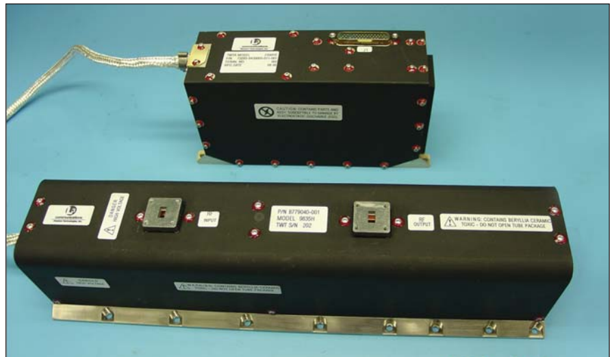
A K-Band 40-W TWTA is shown here for the Lunar Reconnaissance Orbiter Mission.
