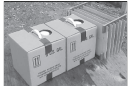
A Bullet Was Fired from the left toward two cubic water-filled containers. The bullet was stopped by the first container.
