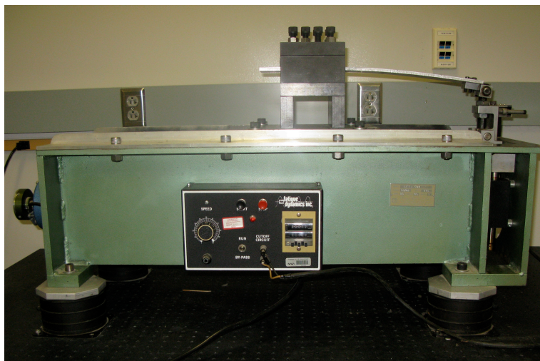
Figure 1: Photograph of the Fatigue Dynamics Inc. Model LFE-500 Life, Fatigue and Endurance Testing Machine with a 0.25 thick aluminum plate in bending.
