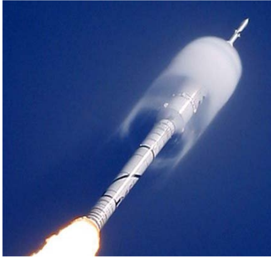
The rocket generated a “halo effect” when moisture was pushed off the front end of the crew module and condensed in the aft air flow.
