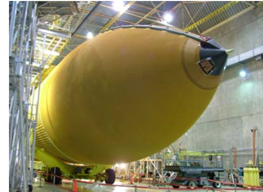
Scissors lifts and stands provide access to all inspection regions except +Z, or top, of tank
