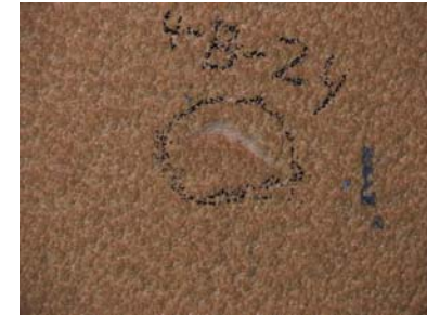
Contamination adjacent to visible impact damage was determined by shearography not to be actual foam damage
