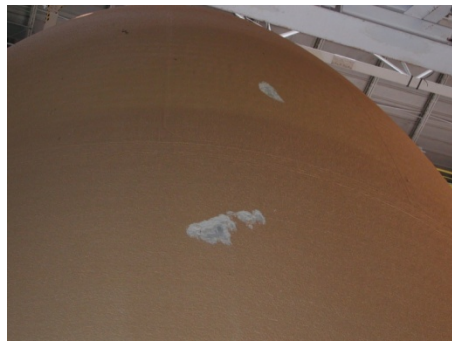
LO2 Tank Ogive Damage
