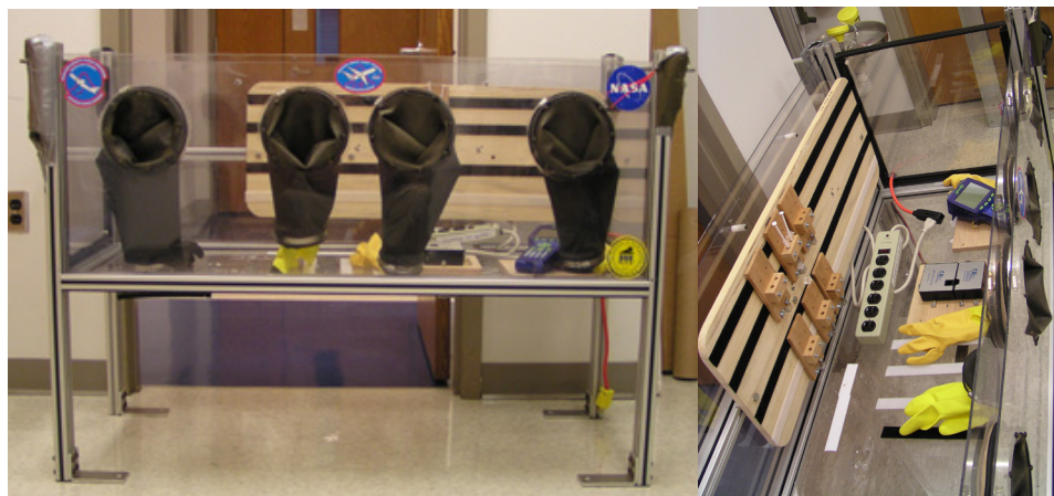
Figure 2. Front and inside view of the double-wall Lexan ® glove box with two sets of industrial-strength rubber gloves. The glove box is shown with video camera mounting bar and top both removed.
