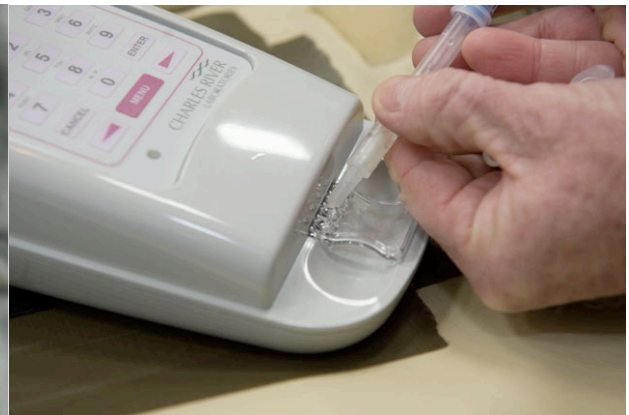
Figure 5. Dispensing droplets into sample wells of a LOCAD-PTS cartridge with the BULB swab unit in zero G. Positioning of the pipette tip 2 to 3 mm from the sample well enabled consistent volumes to be dispensed.
