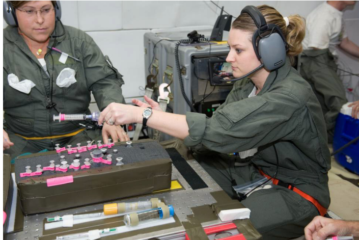
Figure 7. Fluid isolation in medication vial (cap vial adaptor testing).
