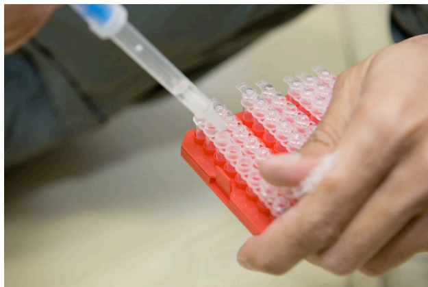
Figure 1. Dispensing droplets into PCR tubes during microgravity. Droplets remained in the tubes because of surface tension and were capped in hypergravity; the volumes were measured on the ground following landing.
