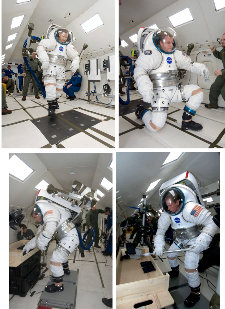
Figure 1. Subjects performing study tasks; clockwise from top left: walking, kneeling and recovering, shoveling, and rock pickup.
