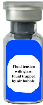
Figure 9. Trapping of fluid in medication vial due to flight adhesion (spike vial adaptor testing).
