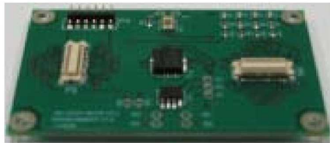
environmental (light, 3-axis accel., temp.)
