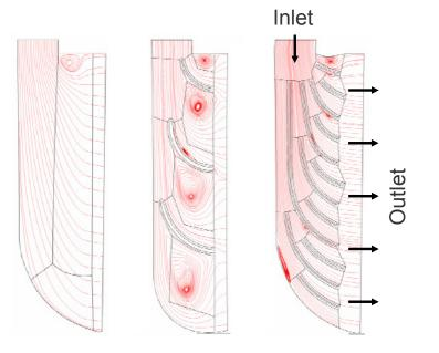
Aerodynamics: loss-minimized flow in plenum of Coanda stator
