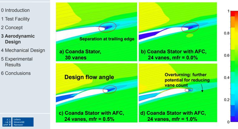
Mach Number Distribution around Trailing Edge at Mid-Span
