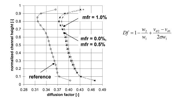
Increased Permissible Aerodynamic Loading by 13% at the Design Point → Better Part Load Performance?
