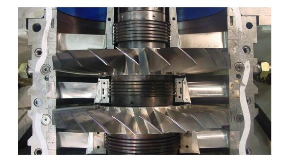
No change of geometry except for Coanda Stator
