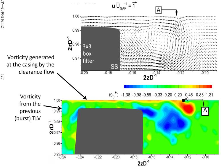
The tip clearance backflow collides with the main flow [point A] inducing a separated flow that follows the TLV outer branch
