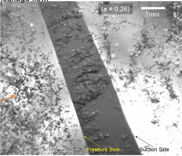
Cloud of bubbles resulting from breakup of vortex generated by previous blade
