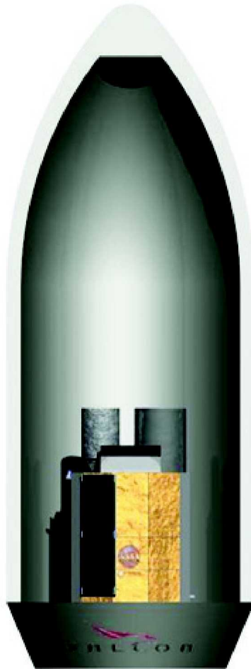
Figure 6. Shroud storage concept.
