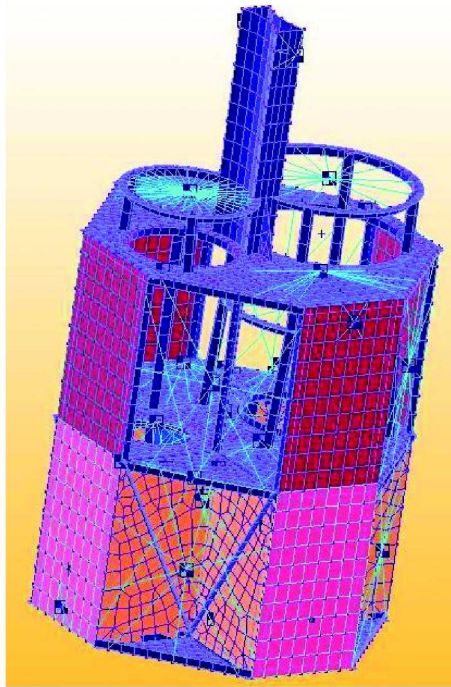
Figure 21. FEMAP FEA model of Xenia spacecraft.
