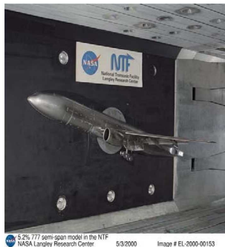
Figure 1. 5.2% 777 Semi-Span Test at NTF (NASA Langley Research Center)
