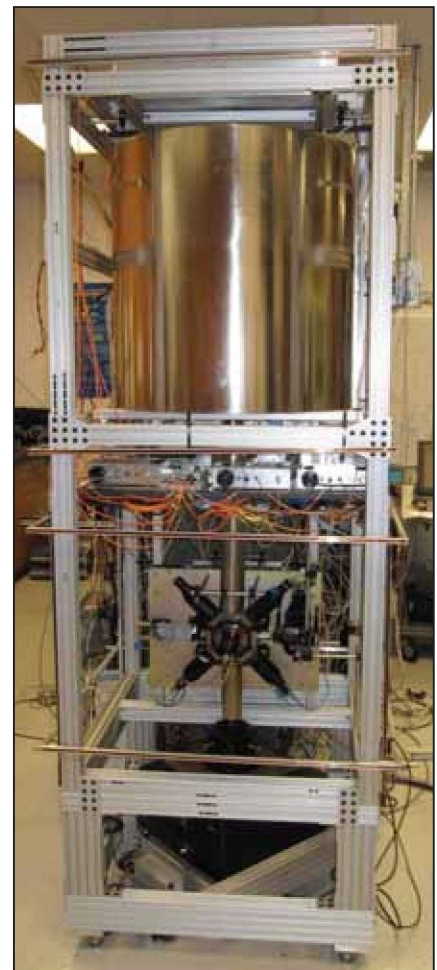
Figure 2. The photograph shows the Quantum Gravity Gradiometer in the laboratory. The magnetic shields around the lower atom interferometer have been removed for clarity.
