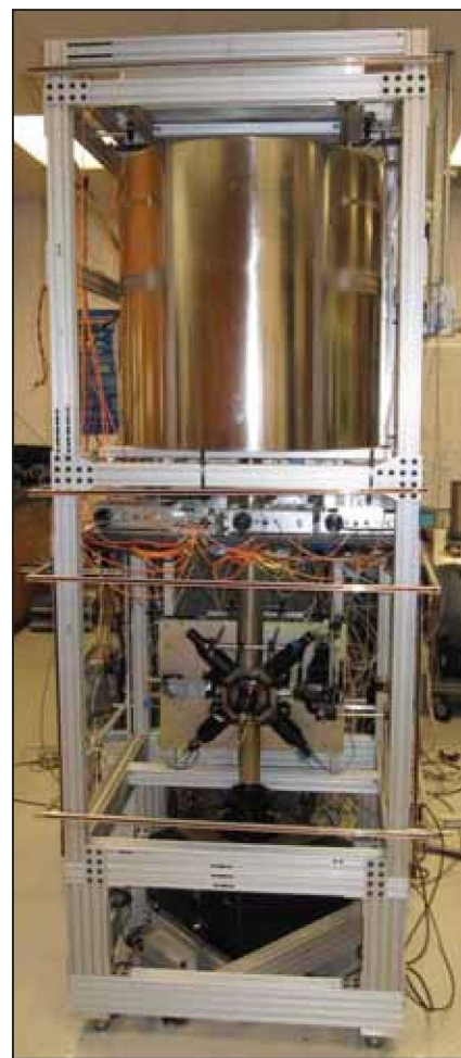
Figure 2. The photograph shows the Quantum Gravity Gradiometer in the laboratory. The magnetic shields around the lower atom interferometer have been removed for clarity.
