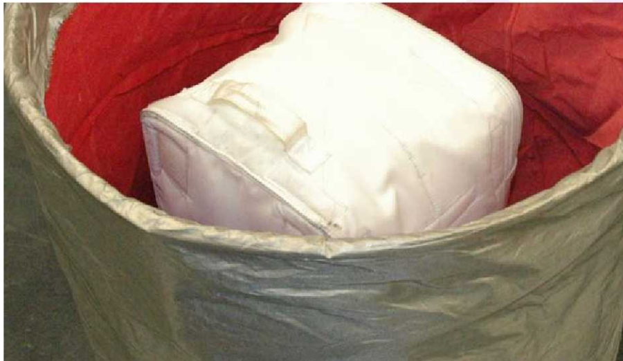
CTB in RFID Enclosure
