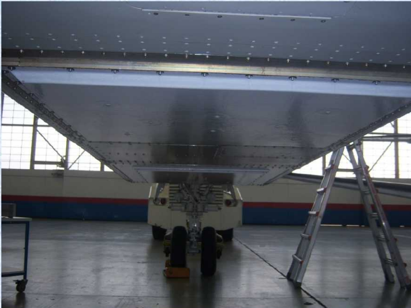
Radar Integrated to P3 aircraft
