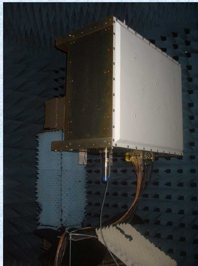
Radar Calibration in Anechoic Chamber
