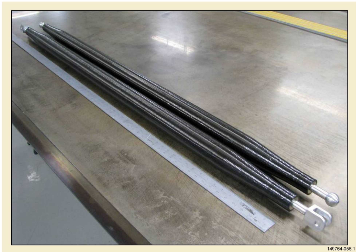
Figure 3.3.1-4. Demo Struts #1 and #2
