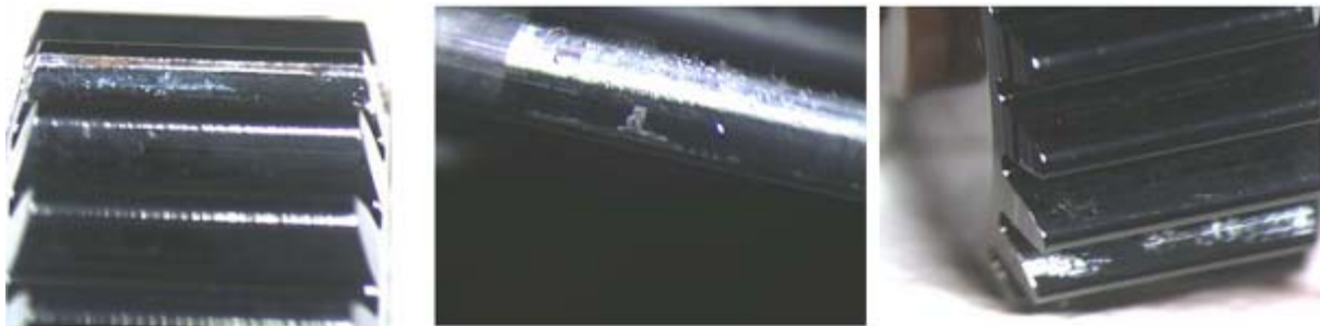
Figure 19: Coating damage after vibration
