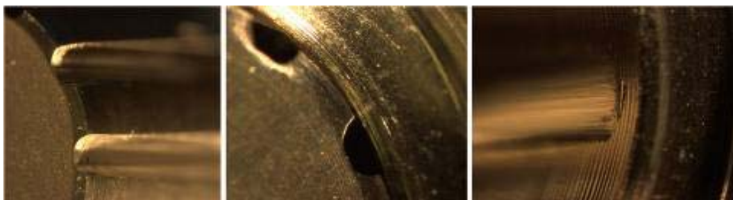
Figure 17: Passed pressing trial results with 40 μm oversize
