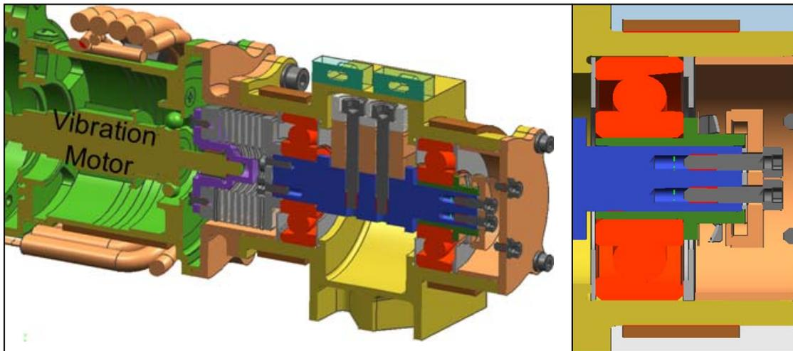
Figure 13. Vibration Mechanism
