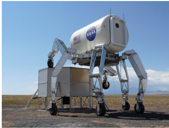
Figure 3. ATHLETE vehicle standing 4-m tall, shown crawling off of a ½ scale lunar lander mockup
