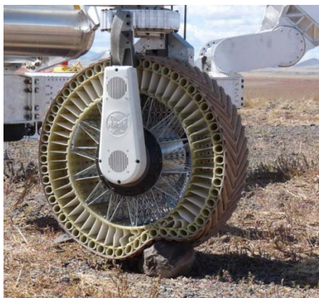
Figure 9. Michelin Lunar Wheel Impacting a 10-cm Tall Rock
