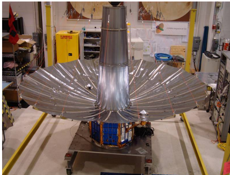
Figure 2: Deployed TacSat-4 UHF Reflector on Comm-X Payload
