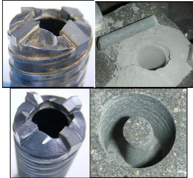
Figure 4. Revision “A” (left) and “B” (right) Coring Bits with Basalt Cores
