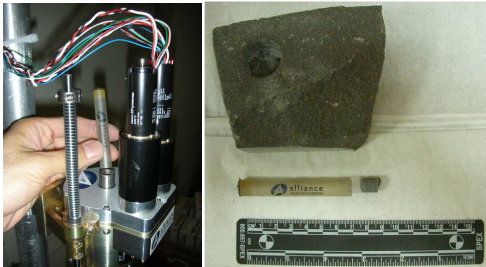
Figure 12. Containment Sleeve at Rear of Integrated Corer (left), Sleeve with Basalt Core (right).
