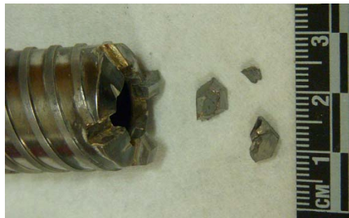
Figure 11. Failed Bit after High Energy Basalt Testing
