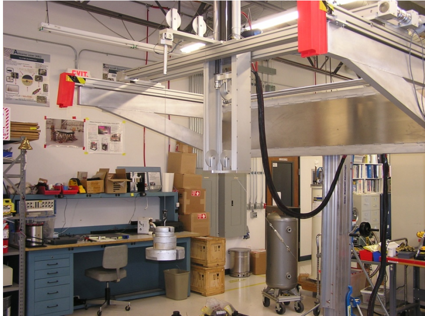
Figure 8: WAGM supporting 360.26-N (80.99-lb) payload
