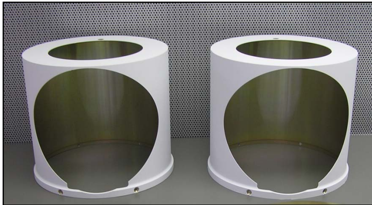
Figure 9. Thermal Baffles Manufactured as Monolithic Structure (Originally Welded)
