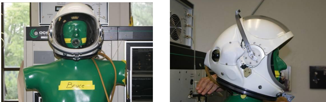
Figure 12: U.S. Air Force S1034 helmet installed on test stand.
