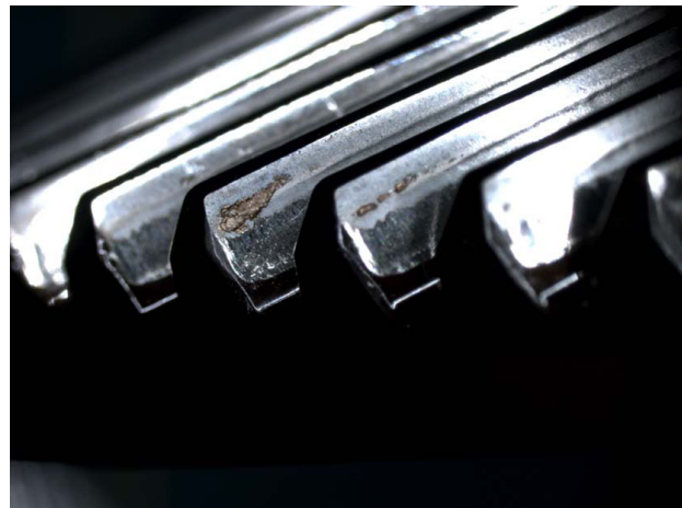
Figure 3. Additional examples of typical gear damage found in the Apache nose gearbox.
