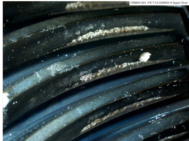
Figure 2. Example of typical gear damage found in the Apache nose gearbox.
