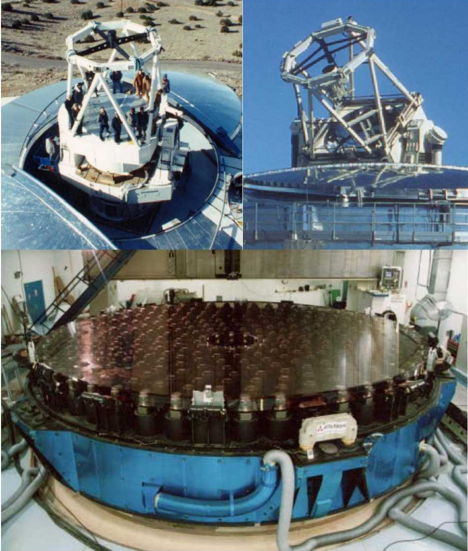
Figure 1 Some large precision optics manufactured by Brashear. (top left) 3.5m Starfire Optical Range telescope. (top right) 3.67m AEOS telescope. (bottom) 8.3m Subaru primary mirror.
