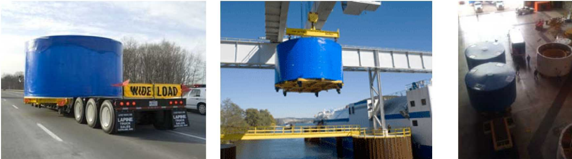
Figure 2. Transport sequence for the Ares I-X Upper Stage Simulator: tractor-trailer to the Ohio River, barge transport on the Delta Mariner to KSC, tractor-trailer from port into the VAB.
