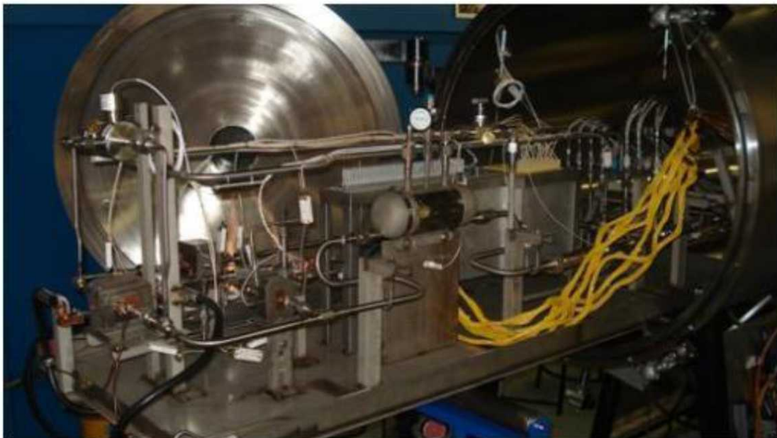
Figure 3. Feasibility Test Loop (FTL) NaK Loading and Verification
