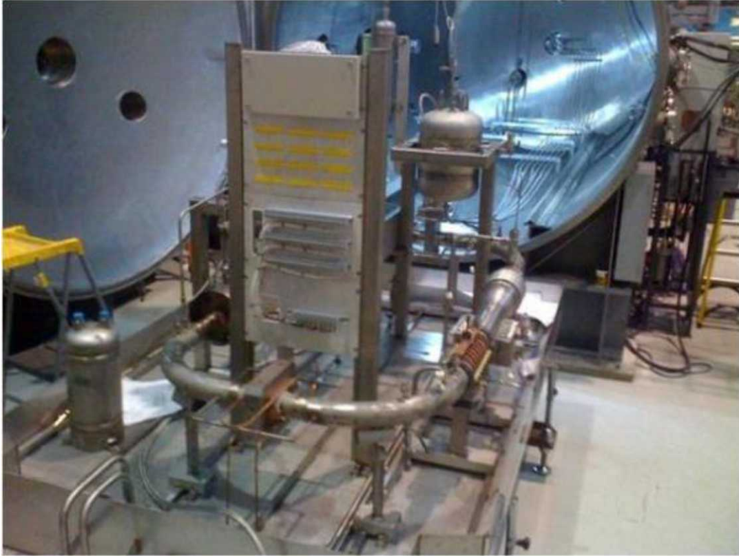
Figure 2. Annular Linear Induction Pump (ALIP) Test Circuit
