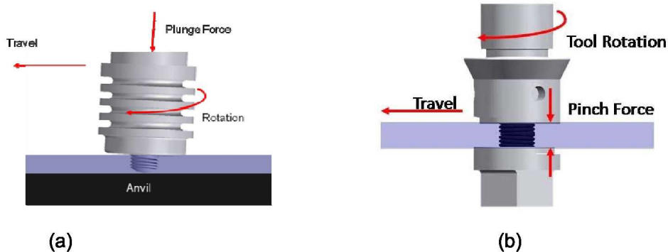
Figure 2. Comparison of conventional (C)-FSW process (a) versus the self-reacting (SR)-FSW process (b). Note the absence of the backing anvil in the SR-FSW process.
