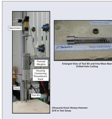
The USROHD Partly Resembles a Twist Drill in that it includes a USDC with a fluted tool bit, rotated by a gearmotor.
